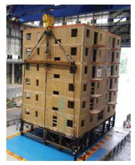
After being lifted to a shake table and subjected to four progressively intense earthquakes, this six-story light-frame building was found to have only minimal damage to the gypsum wallboard and nail connections. (View a video of the test on YouTube.<sup>®</sup>)
