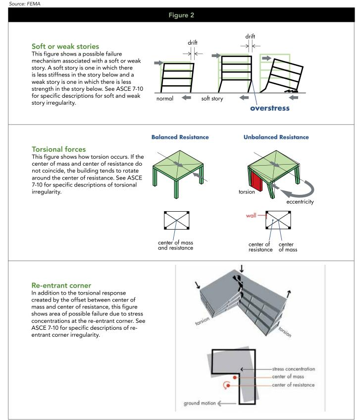
Examples of structural irregularities from FEMA 424 – Design Guide for Improving School Safety in Earthquakes, Floods and High Winds. Another good reference is FEMA 454 – Designing for Earthquakes – a Manual for Architects.
