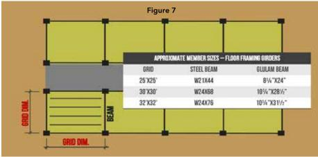
Assumptions: Live load = 40 psf, wood dead load = 30 psf, steel dead load = 70 psf. Sizes shown are for illustration purposes. All member sizes should be provided by a project's structural engineer.
