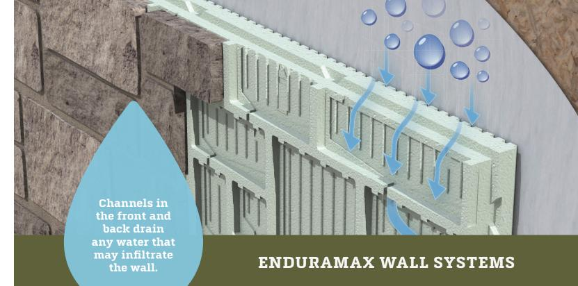
The EnduraMax High Performance Wall System features installation panels that affix to the studs or steel building with stainless steel anchors and screws to provide a framework for several options of brick or manufactured stone veneers.
