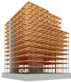
Option 3: Hybrid (Steel Frame with CLT Slab)
