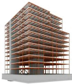
Option 2: Steel Frame (with Composite Slab)
