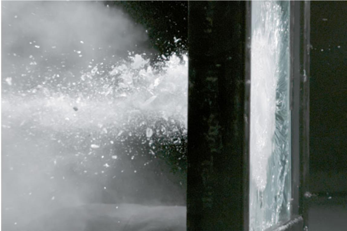
Whether the entire ballistic round or just the fragment create a through-hole in the fenestration assembly, it is a penetration and therefore a failure. By definition, a ballistic threat is the projectile fired from a weapon, and that action may lead to a full or partial penetration of materials. That penetration creates dangers for building occupants, and so must be prevented wherever possible.
