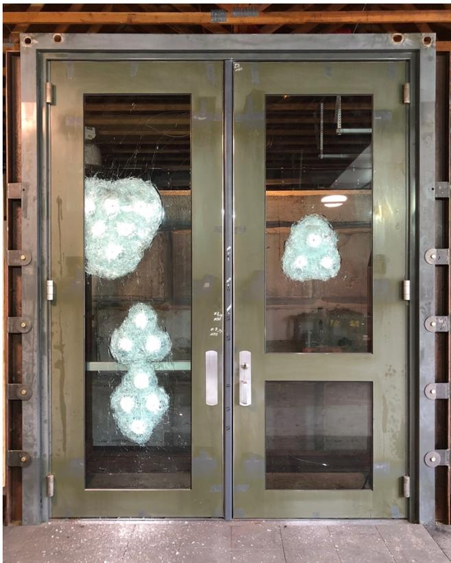
Also a **timed rating**, SD-STD-01.01 has a 5-Minute threat-level rating with no ballistics test, and three others — 15-Minute, 60-Minute, and 15-Minute Fire Rated — with three different ballistic discharge impacts along with attacks by heavy hand tools. When a defined shape can pass through the glazed barrier, a failure has occurred and a
