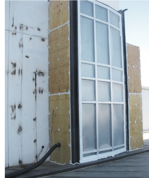
Air Infiltration Chamber (ASTM E-283-04)
