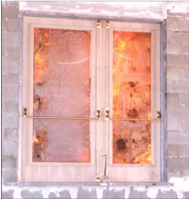
Glass exposed to fire
